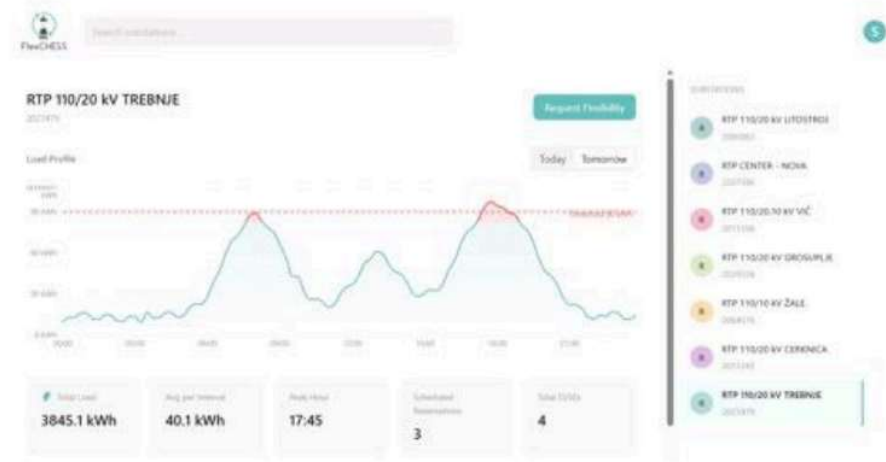
Figure 17: 15-minute interval load profiles for specific substations.
